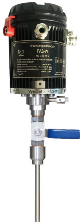
Figure 10. Analyzer FAS-W with a submerged gas supply line without filtration
